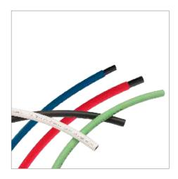
Parflex 95FR MicroWeld™ Tubing is an ideal option for low to medium pressure air and water supply lines where weld spatter protection is required. The double wall design has a flame resistant jacket made from material that meets the UL94 V-0 standard. The specially formulated jacket material is easy to skive back exposing the core tube for quick insertion into Parker's PrestoWeld or PLM fittings.
